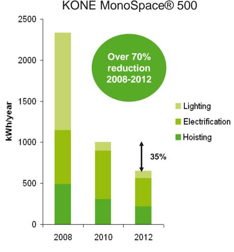
\*The calculation is based on an elevator speed of 1 m/s, a load of 630 kg, 150,000 starts/year, a travel height of 9 m and 4 floors
