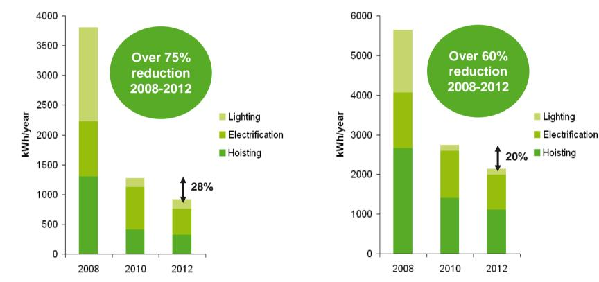
\*The calculation is based on an elevator speed of 1 m/s, a load of 1,000 kg, 150,000 starts/year, a travel height of 12 m and 5 floors
